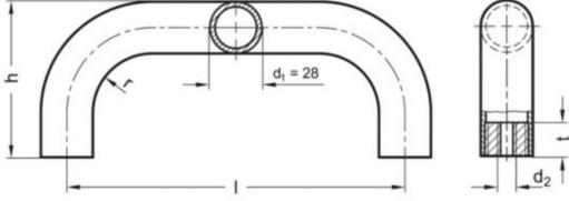
$\begin{array}{ll} d1 &= 20 \\ d2 &= M8 \\ h &= 68 \\ I &= 200 \\ r &= 22 \\ t \min = 15 \end{array}$
